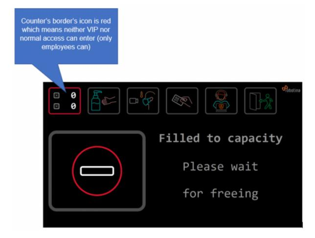
This is the icon that is shown if the alarm is triggered. The border of enter status changes to red. The caption changes to: "Alarm", and the text changes to: "Unauthorized entry, leave immediately".
