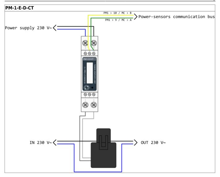
Example of HEMS G2 wiring diagram:
