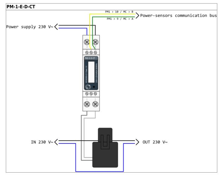
Example of HEMS G2 wiring diagram:
