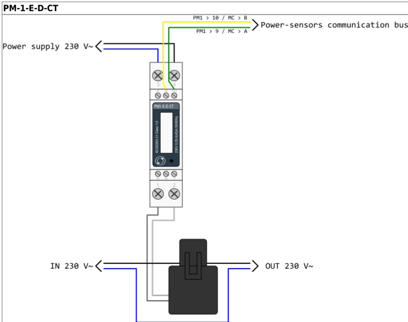
Example of HEMS G2 wiring diagram:
