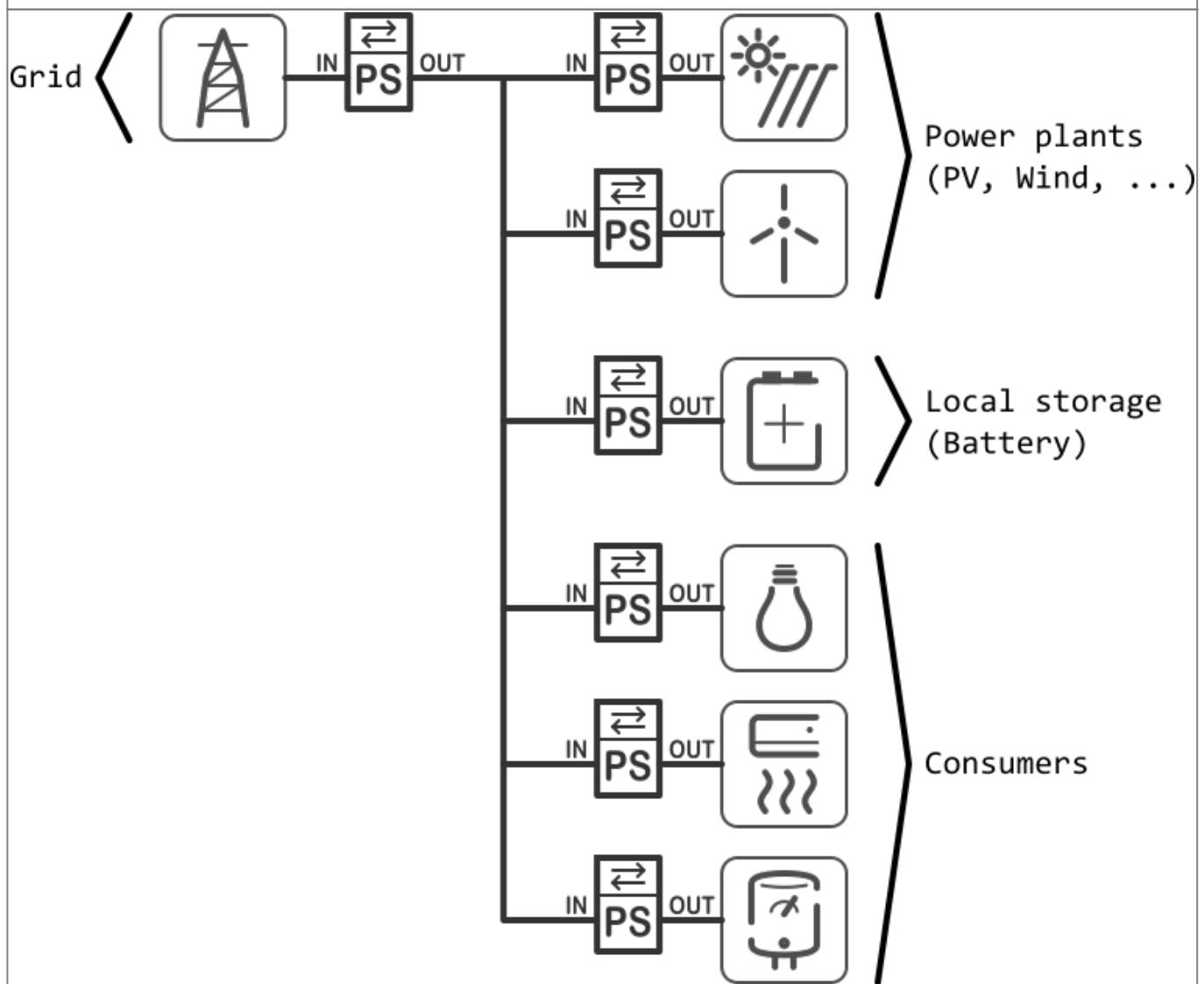
Example of HEMS G2 wiring diagram:
