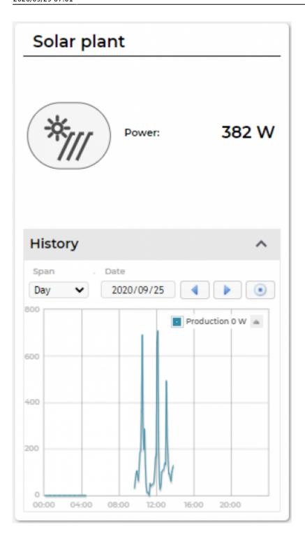
Producers present devices or systems that produce electrical energy. Example of such devices are solar power plant, wind power plant, diesel generator and others. An example on the following figure shows solar power plant.
