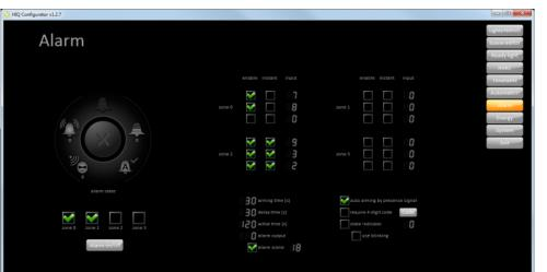
Alarm is based on 4 zones, each with up to 3 sensors. Sensor is configured as number of input where the sensor is connected (0..39). If instant is enabled, alarm is invoked immediately, skipping delay. Arming time is period from turning alarm on to the operative state. Delay time is period from sensor activation to alarm. Active time defines how long alarm output will be active.
