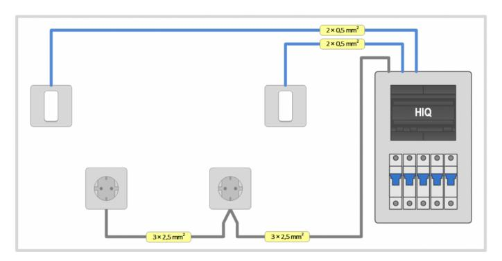
Sockets group is wired to the distribution box with an appropriate wire gauge (usually  $3 \times 2.5 \text{ mm}^2$ )
