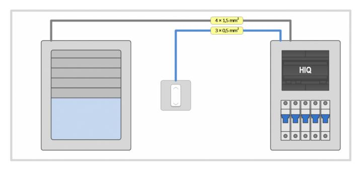
Blind motors are wired directly to the distribution box with an appropriate wire gauge (usually  $4 \times 1.5$  mm<sup>2</sup>)
