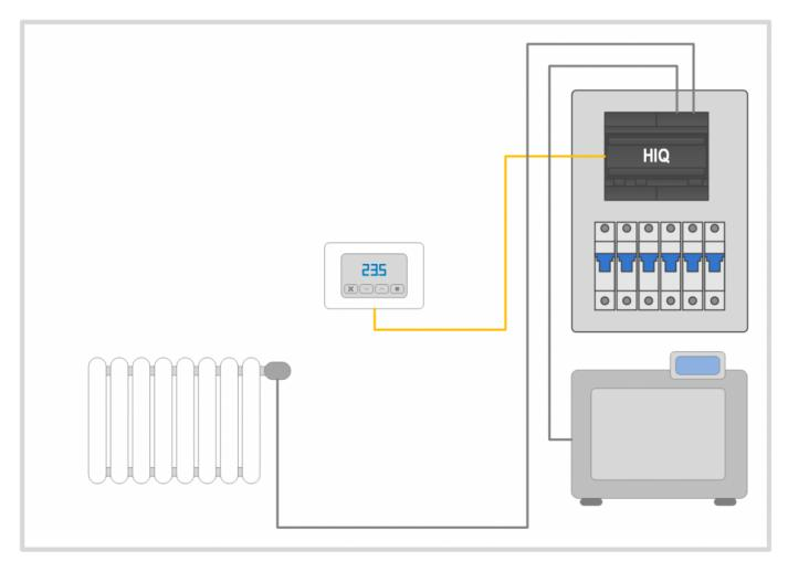
Radiator valves and boiler enable signal are wired directly to the distribution box with an appropriate wire gauge (usually  $3 \times 1.5 \text{ mm}^2$ )
