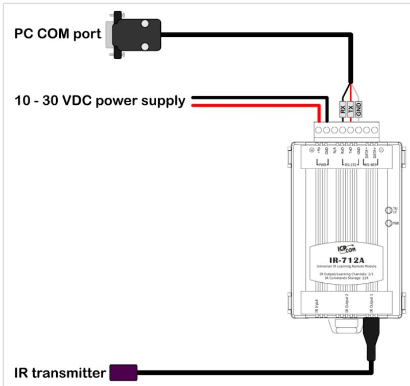
Connect IR blaster IR-712A or IR-210 to power supply and PC.
