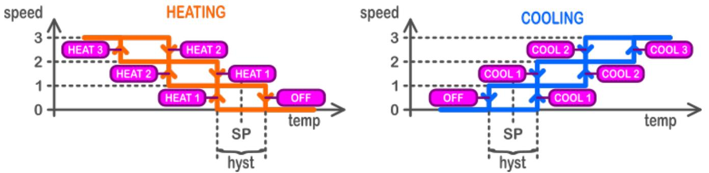
Depending on AC possibilities and user preferences different IR commands for HEAT 1-3 and COOL 1-3 can be used. In the following table there is an example for IR commands for Panasonic inverter AC.
