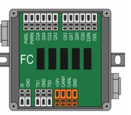
When installing: "Autoaddress" button will link FC-1-IQ unit with lowest serial number with thermostat with lowest serial number and so on.
