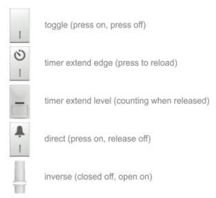
Input mode defines how input affect the output. Basic functions are handled internally by light controller, night mode and ready light are handled with master controller.
