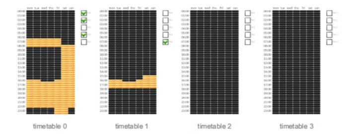
Selected part is a period when heating system is active. Each rectangle represents a half hour. Tables are fully independent of each other. To set multiple fields, hold left button and drag mouse. Each timetable can directly control one output or apply a scene.
