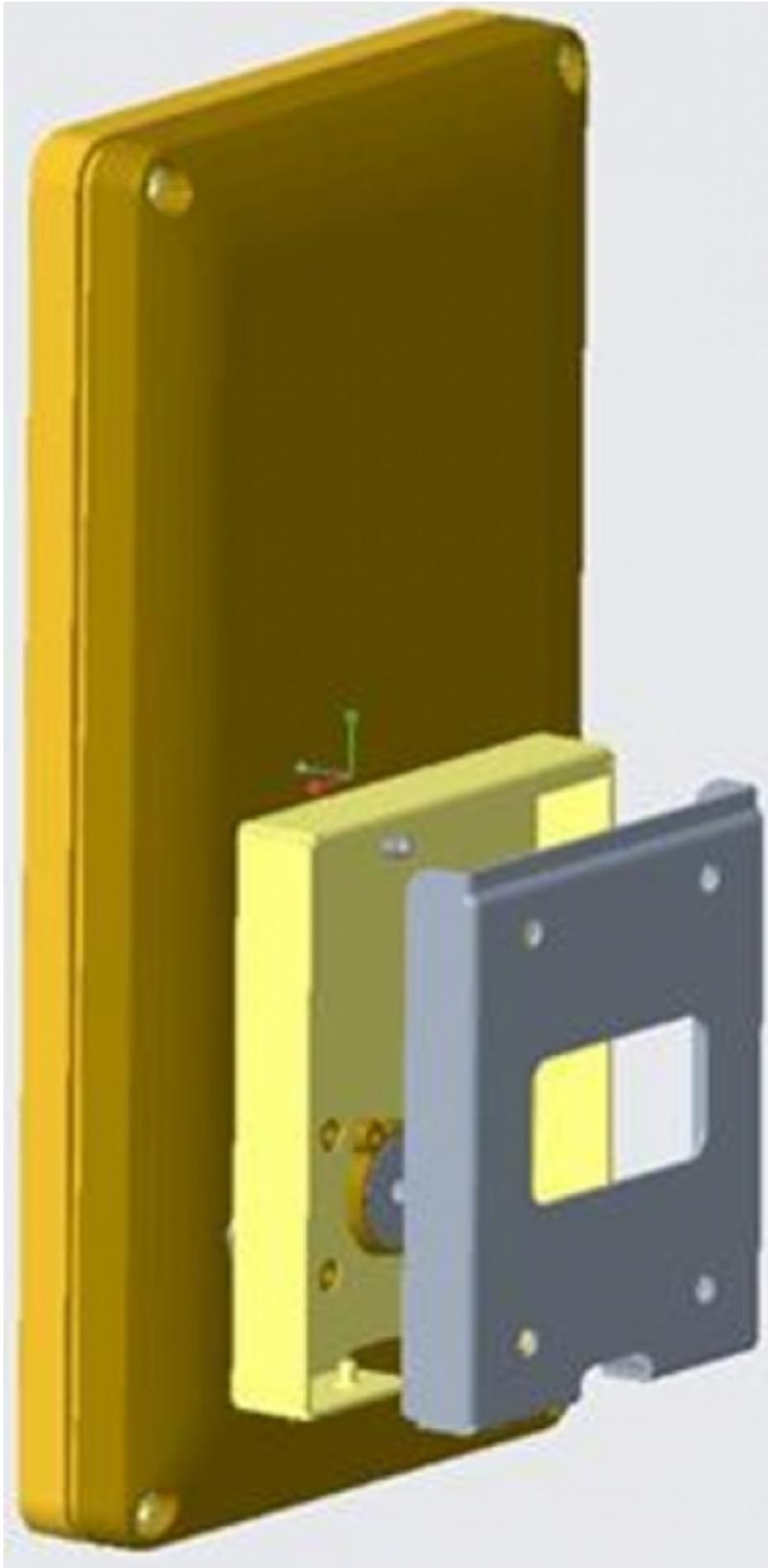
1.After determining the installation height of the device, fix the wall bracket to the wall 2.Insert the corresponding area on the back of the device into the bracket on the wall 3.Align the hole of the wall bracket to hang the unit and pull it down slightly to stabilize it 4.After connecting the wire, tighten the bottom cover with screws.
