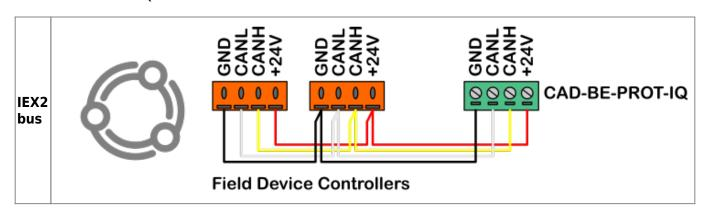
All field modules are connected to the IEX bus with 2 x 2 x 0,8 mm<sup>2</sup> cable.
