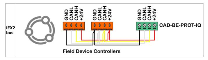
All field modules are connected to the IEX bus with 2 x 2 x 0,8 mm<sup>2</sup> cable.
