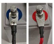
Use the supplied cable with U spade terminals directly for battery/cell wiring
