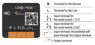
Each terminal can accept a cable of 2.5mm² maximum, stripped of 8mm.
