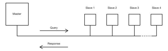
In the MODBUS Protocol the master can address individual slaves, or, using a special "Broadcast" address, can initiate a broadcast message to all slaves. The SDM120CT Digital meter do not support the broadcast address.
