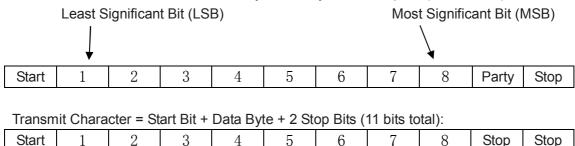
Eastron Digital meters additionally support No parity, 1 stop bit.
